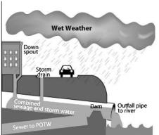
The increase in stormwater costs is primarily to fund new infrastructure that helps protect our rivers by reducing Combined Sewer Overflow, which mixes stormwater with highly polluted wastewater during heavy rain events (see diagram at left).
