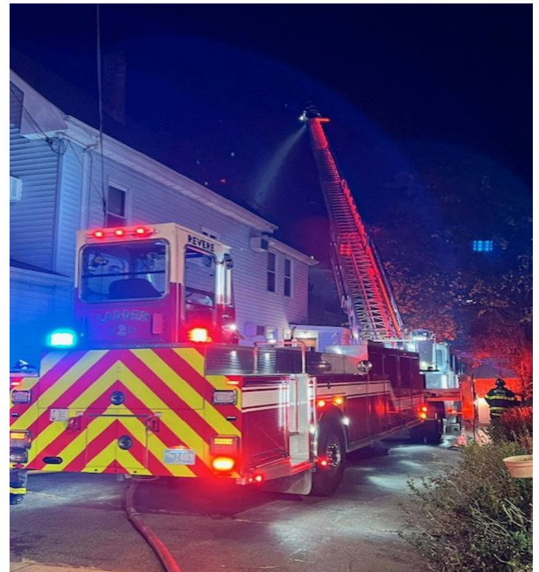
Revere Ladder 2 operating a “ladder pipe” at a multiple alarm fire
